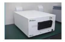
The PCR instrument: It is used for detection of pathogenic microorganism, gene expression level and gene mutation.
